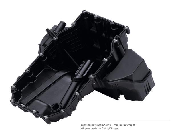
Plastic oil pans offer higher functional integration, less costs and weight in comparison to metallic oil pans. Moreover, bigger volume for the engine's oil is provided which leads to longer service intervals. Various components can be integrated, the complete module reduces the components during the assembly of the engine. Moreover, tailored ribbing structures and appropriate designs improve NVH and stone impact behavior.
