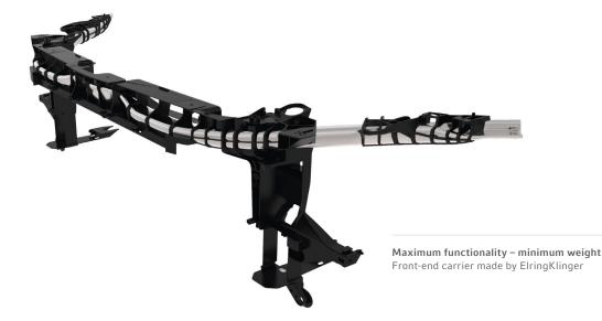
ElringKlinger's structural front-end carrier produced as a hydroforming hybrid design can serve as a support for the intercooler, headlight modules, windscreen wiper water reservoir, horn, distance radar module or air intake. It also supports the bonnet.
