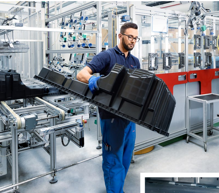
Plastic oil pans from ElringKlinger offer significant potential for weight and cost savings, for example in the commercial vehicles sector.
