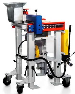
The mechanical press can exert seven metric tons of pressure. It produces a clay brick in just four minutes.
