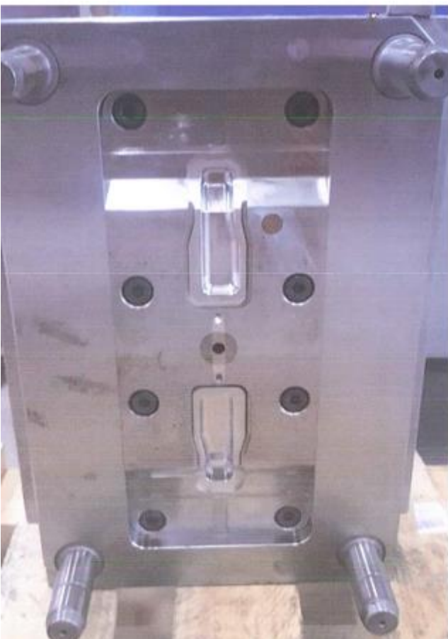
Example pictures of opened two cavity tool.
